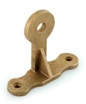
Rod brackets are made of copper alloy. Rod bracket being used for providing projection from building or face. Rod bracket is mainly used with rod to tape coupling where it is not possible to fit saddle on the roof and theair rod has to be fitted on the side of the building.
