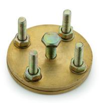
Plate type test clamp are used as T Joint or straight through joints of tapes. It is also used for testing points for the network by disconnecting the joints. These also used for heavy duty tape up to 50x6 tape.
