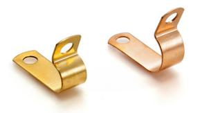
One hole cable clip are made from copper sheet. This is used to fix conductor to structures. The clip is fixed to the structure with wood screw.
