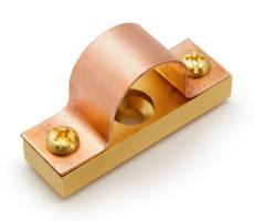
Circular Conductor Clip are made of copper alloy. The clip has a hole in the base for fixing with building or structures with appropriate screw and wall plug. These are used to secure copper conductor the building or structures.
