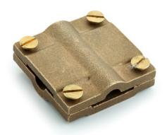
These are made from gunmetal or brass.These clamp are used for crossing over tapes and cable. To make straight through joint or T connection in a continues network.The lids are secured by four screw.
