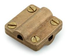
Square conductor clamp are made from gunmetal or brass these are used for 4 way connection straight or T joints for round conductors. The lids are secured by four screw.
