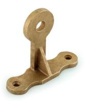
Rod brackets are made of copper alloy. Rod bracket being used for providing projection from building or face.Rod bracket is mainly used with rod to tape coupling where it is not possible to fit saddle on the roof and theair rod has to be fitted on the side of the building.
