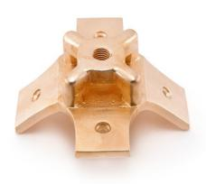
Ridge saddle are made of gun metal or brass. Used for vertical support to lightening conductor air terminal on the roof edges. These are used for fixing air rod and connecting to tape.
